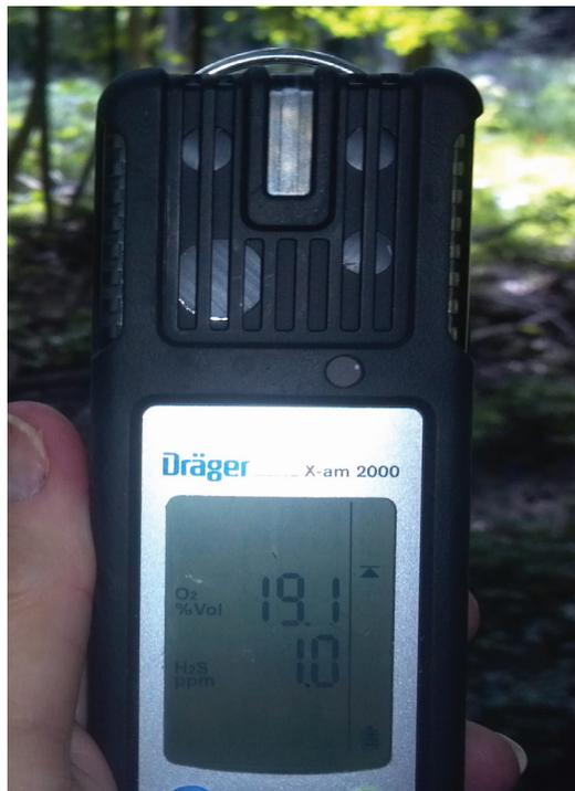
August 9, 2013 – Dräger 2000 Oxygen and Hydrogen Sulfide air meter registers 19.1 % O<sub>2</sub> and 1.0 ppm H<sub>2</sub>S (1 ppm = 1,000 ppb) at property next to Hartland Farms liquid manure spray-application in Hudson Twp, Lenawee Co., Michigan.
